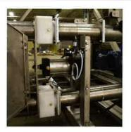
Spiroflow's patented Dynamic Automatic Rope Tensioner (DART) extends rope life by up to 40% and decreases maintenance costs.
