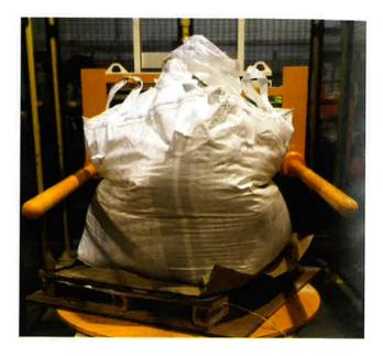
Spiroflow's bulk bag conditioner easily and effectively breaks up solid ingredient contained within bulk bags. Depending on your material it may require only two or three 'squeezes' to do the job.
